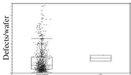
Figure 6. InP layer defectivity of InP-on-GaAs engineered substrate as seen by Candela before epitaxy for a layer transfer from a fresh bulk InP wafer (baseline) and bulk InP wafer recycled 7 times.
