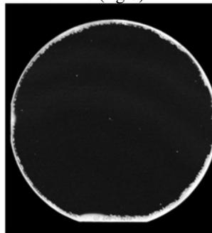
Figure 8. SAM image of a 100 mm diameter sample with four-junctions bonded built on top of an InP-on-GaAs engineered substrate.
