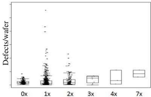
Figure 5. InP bulk defectivity as seen by Candela as a function of refresh cycles. The data at 0x corresponds to fresh InP.
