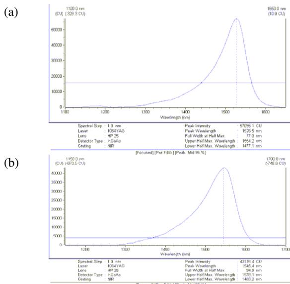
Figure 10. Photoluminescence wavelength distribution of a 1.55µm MQW structure grown by GSMBE epitaxy respectively on bulk InP (a) and InP-on-GaAs (b)
