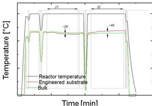
Figure 7. Comparison of in situ temperature monitoring (wafer temperature) during epitaxy growth of GaInAs (J1) and GaInAsP (J2) on bulk InP and InP-on-GaAs (engineered substrate).
