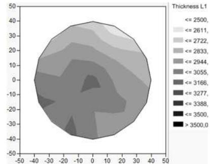
Figure 4. 100mm wafer with thin InP transferred film on GaAs. Thickness is expressed in Angstroms as measured by spectroscopic ellipsometry.
