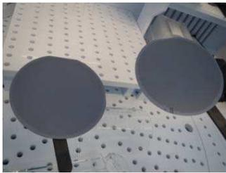
Figure 2. 100mm wafer with thin InP transferred film on a new support substrate (GaAs in this case) following Smart Cut™ technology on the left. Remaining InP wafer is on the right ready for recycling
