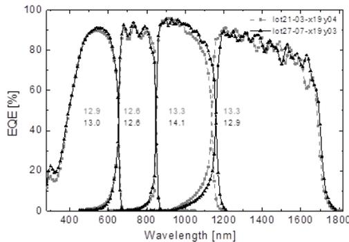
Figure 9. Comparison of external quantum efficiencies for a 4-junction cell grown on a InP bulk substrate (wafer 21-03) or a InP-on-GaAs engineered substrate (wafer 27-07).
