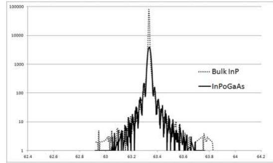
Figure 3. Comparison of XRD rocking curves of InP bulk material and InP-on-GaAs engineered substrate.
