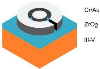
Figure 2: Physical layout of planar MOSCAP structures fabricated on III-V substrates, showing the layer stack of each device.
