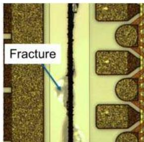
Figure 3. Subsurface fracturing due to higher dicing speed.
