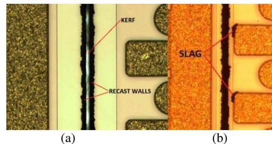
Figure 9. Optical images of laser dicing street and defects. (a) With slow coat speed; (b) with high coat speed.
