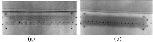
Figure 12. X-ray images on assembled die from laser saw process. (a) Solder voids (white spots) are apparent from initial laser saw process. (b) No solder voids are seen from final laser saw process.
