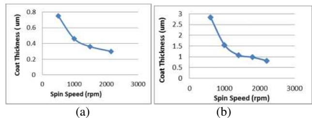
Figure 8. Coat thickness as a function of spin speed for the first type of coat (a) and the second type (b).
