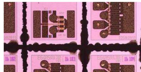
Figure 10. Optical image of blowout defect from laser dicing with coat inadequately cured.
