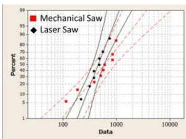
Figure 11. Probability plot of FET DC lifetime comparing mechanical saw and laser saw.
