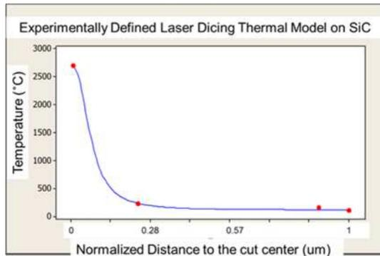
Figure 7. Experimentally defined temperature during laser dicing as a function of the distance from the center of the dicing street.
