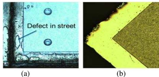
Figure 13. Optical images of street defects from mild adhesion tape (a) vs strong adhesion tape (b)
