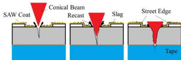
Figure 1. Ablation laser dicing process.
