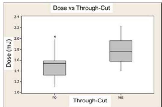
Figure 5. Laser pulse dose vs. through cut.
