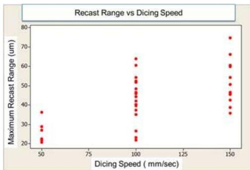
Figure 2. Recast range vs laser dicing speed.
