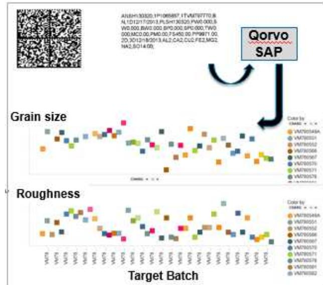
Figure 1: The Metal supplier provides certificate of analysis (COA) data into a 2D bar code. The receiving department scans the bar code and the data is uploaded to SAP® where it can be accessed by Spotfire® for display, correlations etc.
