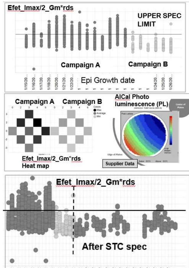
Figure 5: (Top to bottom) 1. Epi Campaign A was failing for an RF test parameter. 2. RF parameter Heat Map for Campaign A showed a strong Northeast to Southwest signature indicative of MBE reactor and similar to the map of Schottky Aluminum % variation across the wafer. 3. Al% Standard deviation Upper Control Limit was added to the STC spec and RF test failure was eliminated.
