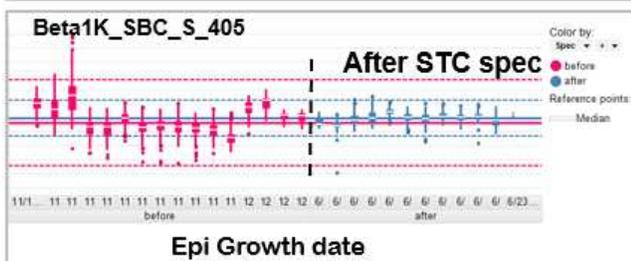
Figure 6: From top to bottom- 1. Yield engineering investigated yield fallout at final test due to low beta and found correlation to the wafer edge of particular epi runs. 2. The supplier collects data at various sites and was able to predict the low Beta. 3. Beta Range and Min was added to the STC spec. 4. The failure mode was eliminated.
