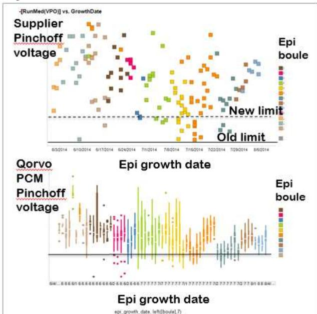
Figure 4: The supplier pinch off voltage (top) for one of our pHEMT epi showed a trend down but was still within our original ship to control spec. Qorvo device voltage (bottom) trended low and started failing the spec limit. We worked with the supplier to implement a new STC limit (dotted line, top) and eliminated the failures.
