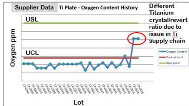
Figure 3: Oxygen (ppm) in Titanium target. The supplier caught the uptick as part of Ship to Control and found out that there had been a change in the Titanium powder supply chain. The Ti powder source had increased the ratio of revert/crystal Ti due to an issue with the Titanium sponge. The new ratio was considered qualified by the raw material supplier and the material in spec, therefore they had not notified our target supplier.
