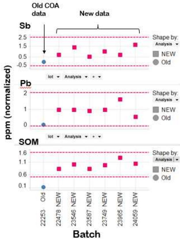
Figure 2: Antimony, lead and Sum of Metallics (SOM) in a tin material. The supplier historical COA (circle marker) was inconsistent and did not align with an independent analysis we had done on the material due to an excursion. The supplier engaged a different lab and started reporting data in alignment with the independent analysis (square markers). The dotted lines and +/- 3 sigma for the square datapoints.
