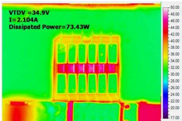
Figure 5-IR temperature measurement of GaN-on-Diamond resistor mounted to micro-channel cooler
