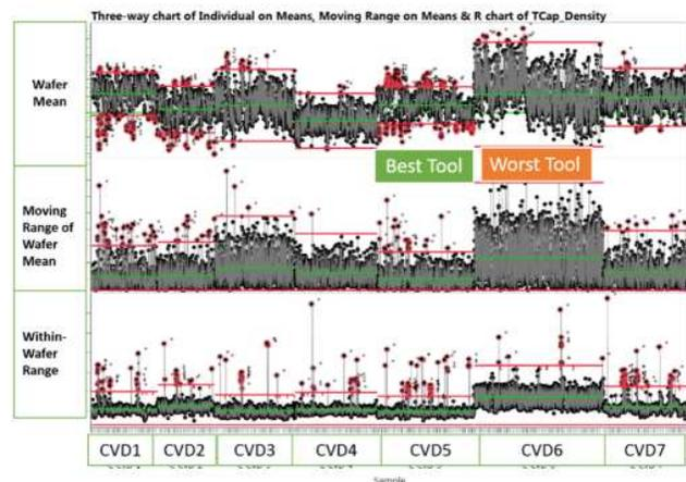
Figure 2. Capacitance density wafer mean, moving range, within-wafer range comparison for wafers processed on different CVDs.
