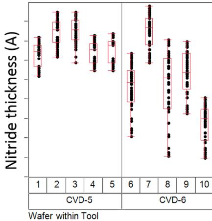
Figure 3. Nitride thickness difference for 5 wafers in a batch processed on CVD5 and CVD6.
