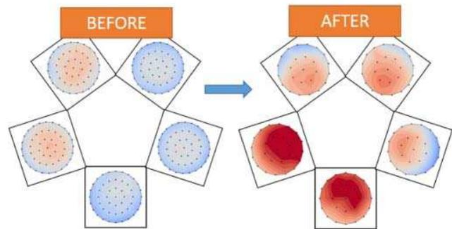
Figure 6. CVD5 (the best tool) nitride deposition thickness before and after swapping showerhead with CVD6.
