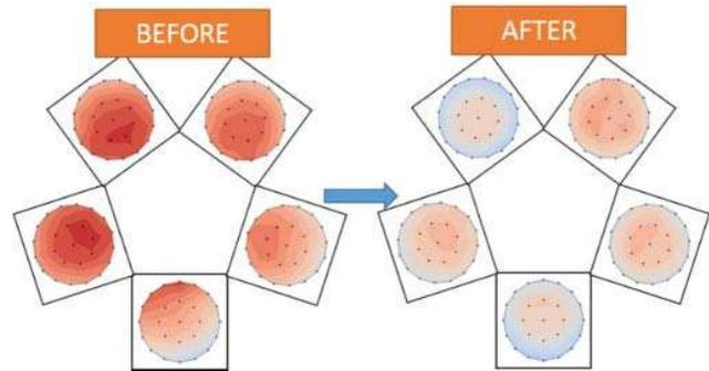
Figure 5. CVD6 (the worst tool) nitride deposition thickness before and after swapping showerhead with CVD5.
