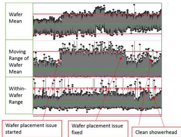
Figure 4. Nitride thickness trend with different tool activities on CVD6.
