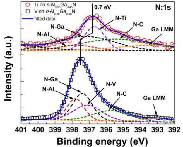
Figure 5. XPS spectra of N:1s core level at the annealed V-Al<sub>0.55</sub>Ga<sub>0.45</sub>N and Ti-Al<sub>0.55</sub>Ga<sub>0.45</sub>N interfaces. The N:1s core level was fitted using Shirley background and mixed Lorentzian-Gaussian line shapes.
