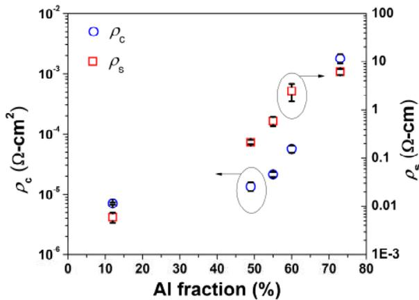
Figure 4.  $\rho_c$  and  $\rho_s$  of V/Al/Ti/Au ohmic contact on  $n\text{-Al}_x\text{Ga}_{1-x}\text{N}$  films with various Al compositions ( $x=0.06, 0.49, 0.55, 0.6,$  and  $0.73$ ).
