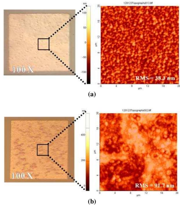
Figure 2. The microscopic and AFM images for the annealed (a) V/Al/Ti/Au and (b) Ti/Al/Ti/Au metal stacks.
