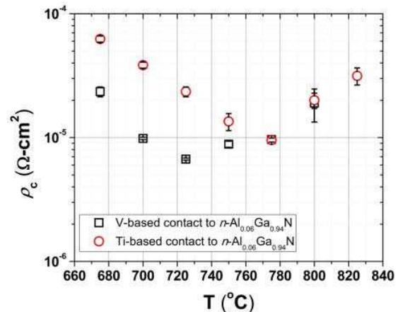
Figure 3.  $\rho_c$  of V/Al/Ti/Au and Ti/Al/Ti/Au ohmic contact as a function of annealing temperature on Al<sub>0.06</sub>Ga<sub>0.88</sub>N film.
