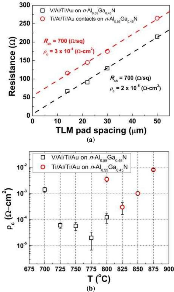
Figure 1. (a) TLM results of V/Al/Ti/A and Ti/Al/Ti/A ohmic contact on Al<sub>0.55</sub>Ga<sub>0.45</sub>N film. The V-based ohmic contact was annealed at 775 °C for 1 minute in N<sub>2</sub>. The Ti-based ohmic contact was annealed at 825 °C for 1 minute in N<sub>2</sub>. (b)  $\rho_c$  as a function of annealing temperature for V/Al/Ti/Au and Ti/Al/Ti/Au ohmic contact on Al<sub>0.55</sub>Ga<sub>0.45</sub>N film.
