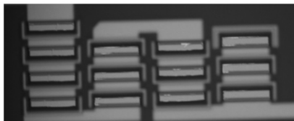
Figure 3: On-mesa metal damage caused by MLO process, described as Pattern Bright defects.
