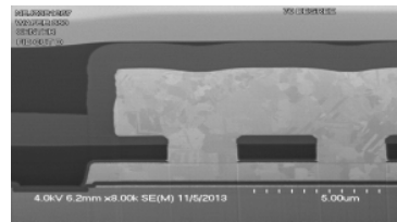
Figure 10. Integration of a secondary low stress SiN on BCB with ALT4F multi-layer final passivation [4].
