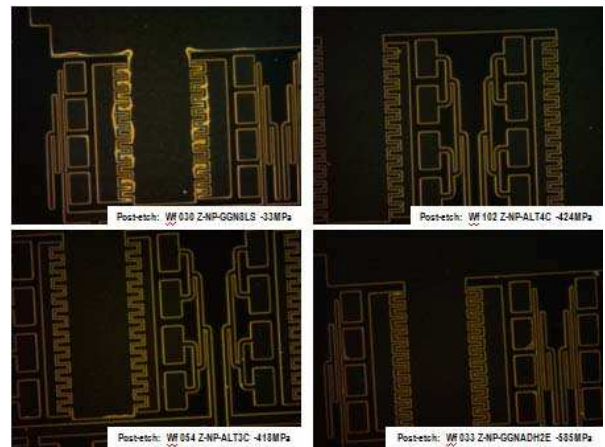
Figure 8. A KII etch for 1 hour shows the low stress GGN films seriously attacked, whereas highly compressive films are not attacked.
