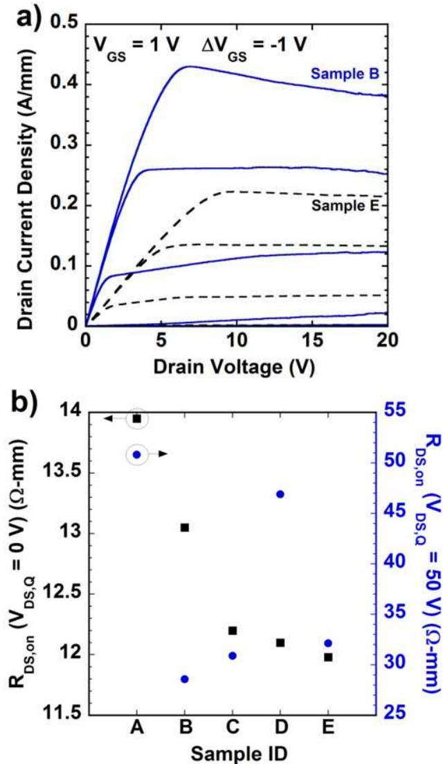
Fig. 2. a) Comparison in DC  $I_{DS}$ - $V_{DS}$  characteristics for samples B and E. b)  $R_{DS,ON}$  as a function of 0 V and 50 V quiescent drain-source bias for samples A-E.
