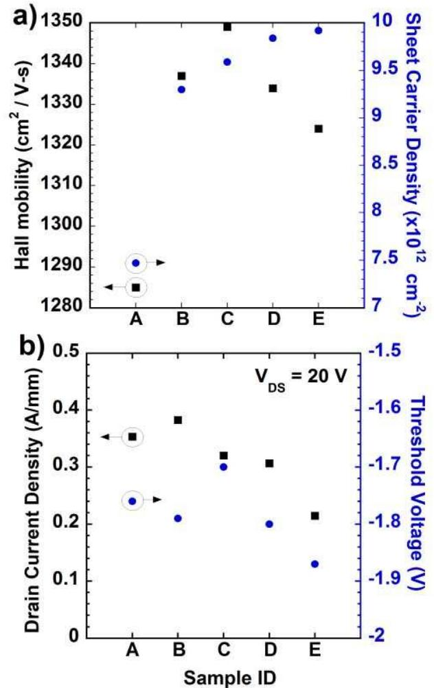
Fig. 1. a) Hall mobility ( $\mu_H$ ), sheet carrier density ( $N_{SH}$ ), b) saturation drain current density ( $J_{DS,SAT}$ ), and threshold voltage ( $V_{TH}$ ) for samples A-E.
