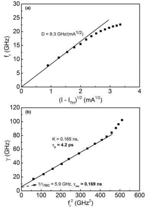
Figure 4. (a) Resonance frequency vs.  $\sqrt{I - I_{TH}}$  graph. The fitted slope of the data points is the D-factor. (b) Damping rate vs. resonance frequency graph for different biasing points. The extracted photon lifetime, from the inverse of the slope, is 4.2 ps and the extracted recombination lifetime, from the intercept, is 0.169 ns.
