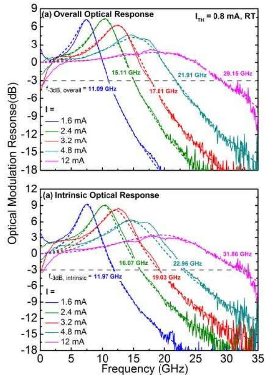
Figure 3. (a) The overall optical frequency response and (b) the intrinsic optical response of the modeled 5  $\mu\text{m}$  aperture. The highest - 3dB modulation bandwidth of the overall optical response is 29.15 GHz whereas it is 31.86 GHz for the intrinsic optical response.
