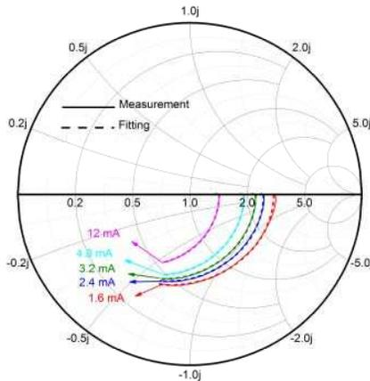
Figure 2. Measurement data and fitting of the electrical reflection coefficient of our 5  $\mu\text{m}$  aperture 57 Gb/s error free VCSEL. The fitting curves are generated from the equivalent circuit shown in Fig 1. Various electrical parasitic parameters are shown in Table I.
