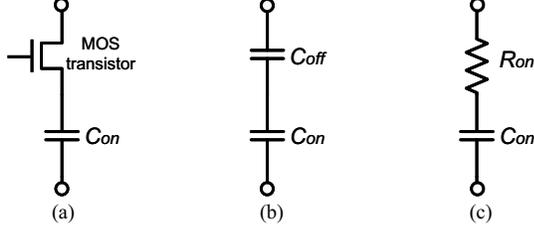
Fig. 2. (a) Schematic of a capacitive switch composed by a series connection of a fixed capacitor ( $C_{on}$ ) with a MOS transistor. (b) Equivalent circuit of the capacitive switch in the OFF state. (c) Equivalent circuit of the capacitive switch in the ON state.
