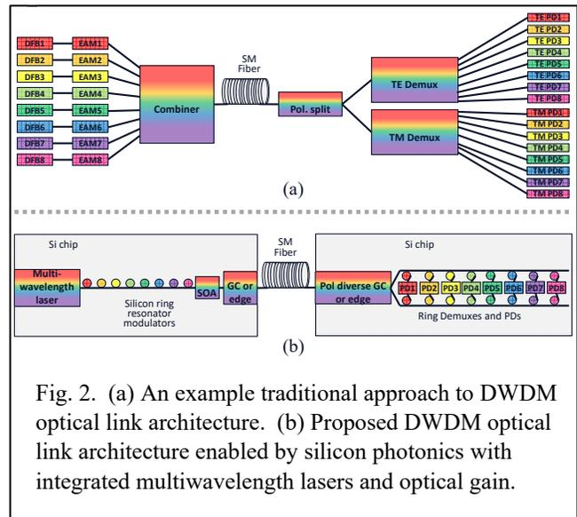
Fig. 2. (a) An example traditional approach to DWDM optical link architecture. (b) Proposed DWDM optical link architecture enabled by silicon photonics with integrated multiwavelength lasers and optical gain.
