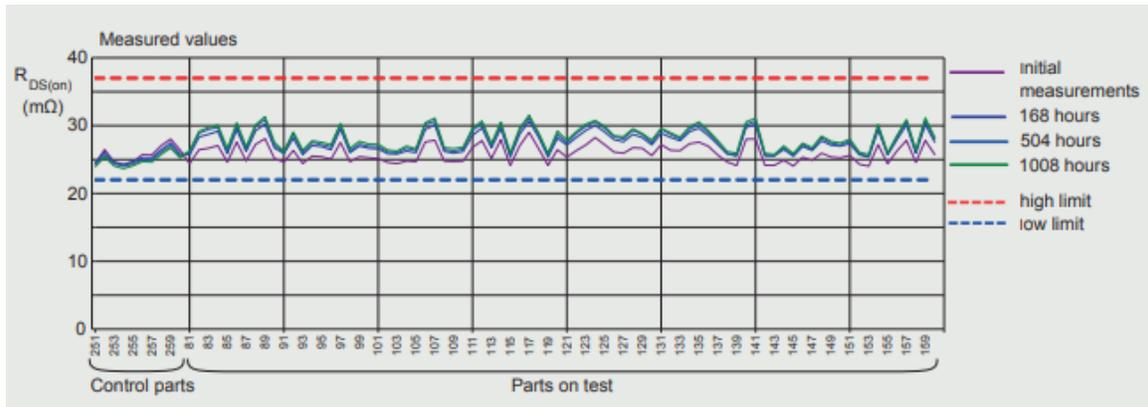
Fig. 4. Dynamic  $R_{DS(on)}$  measurements during HTRB.
