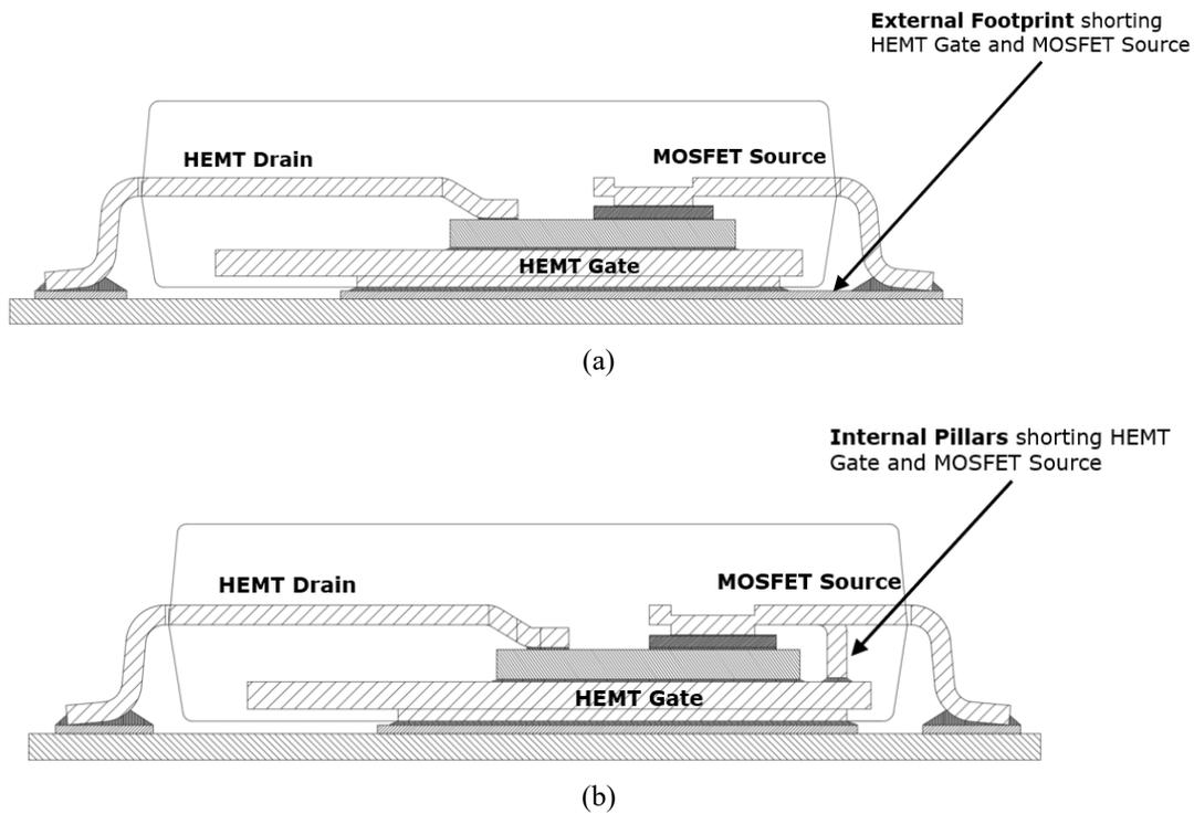
Fig. 2. – External (a) and Internal (b) connection between the gate of the HEMT and the source of the MOSFET (the usual cascode connection) in the bottom cooled devices. Nexperia is introducing option (b).
