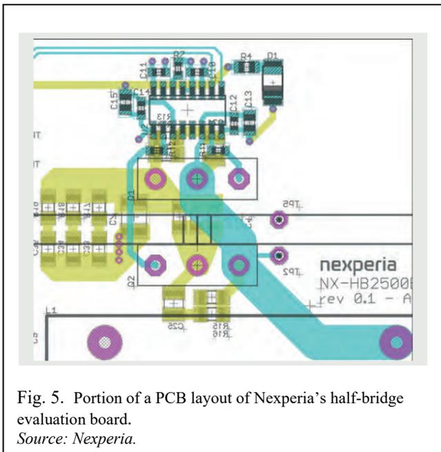
Fig. 5. Portion of a PCB layout of Nexperia’s half-bridge evaluation board.
