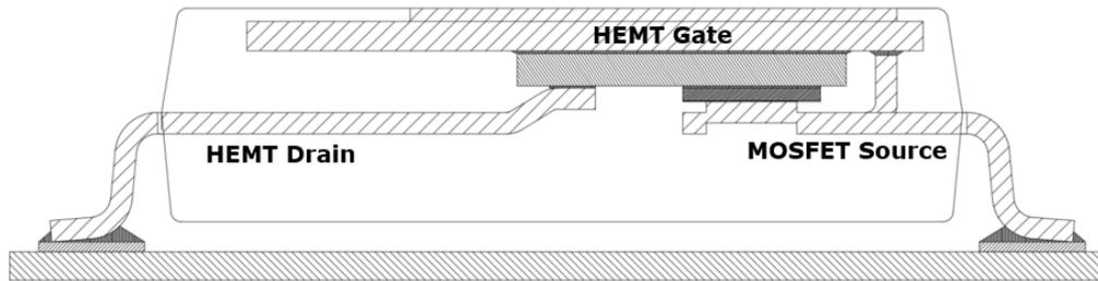
Fig. 3. Top side cooled CCPAK1212.
