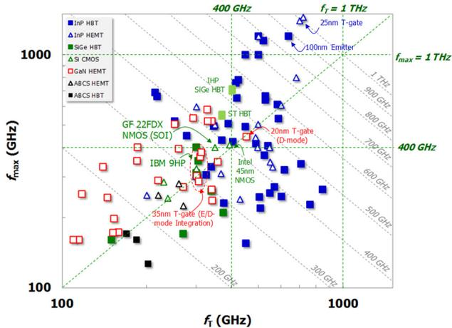
Figure 2: State-of-the-art transistor speed for multiple compound semiconductors and Si CMOS.
