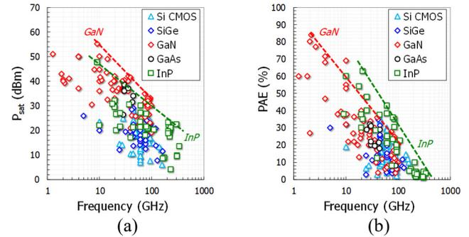
Figure 3: RF MMIC output power and Power Added Efficiency (PAE) for multiple compound semiconductors and Si CMOS.
