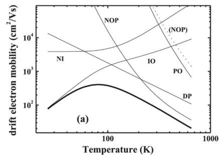
Figure 4: Simulated drift mobility of  $\beta$ -Ga<sub>2</sub>O<sub>3</sub> versus temperature. (Figure courtesy of A. Parisini and R. Fornari, University of Parma, and IOP Publishing [2].)
