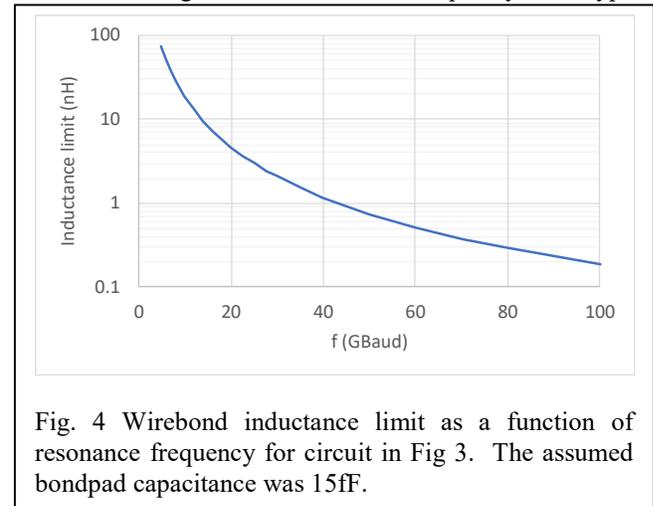
Fig. 4 Wirebond inductance limit as a function of resonance frequency for circuit in Fig 3. The assumed bondpad capacitance was 15fF.
