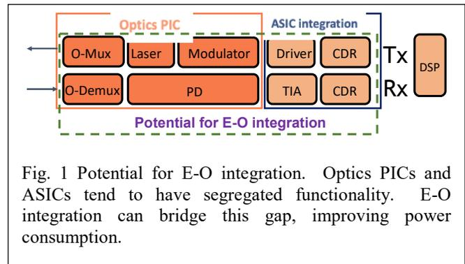
Fig. 1 Potential for E-O integration. Optics PICs and ASICs tend to have segregated functionality. E-O integration can bridge this gap, improving power consumption.
