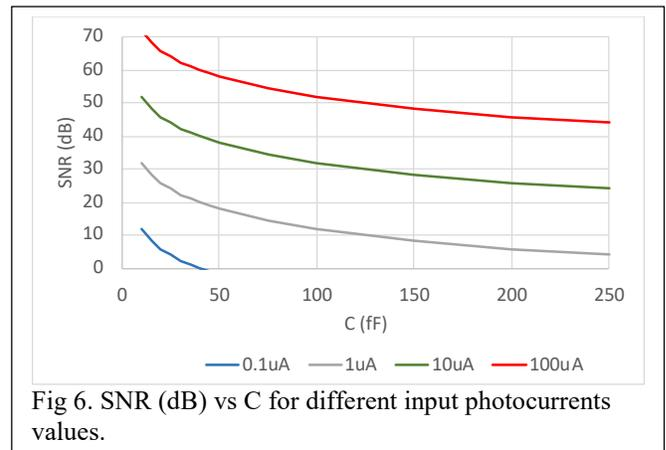
Fig 6. SNR (dB) vs C for different input photocurrent values.
