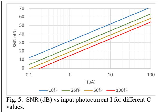
Fig. 5. SNR (dB) vs input photocurrent I for different C values.
