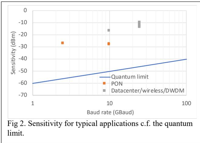
Fig 2. Sensitivity for typical applications c.f. the quantum limit.
