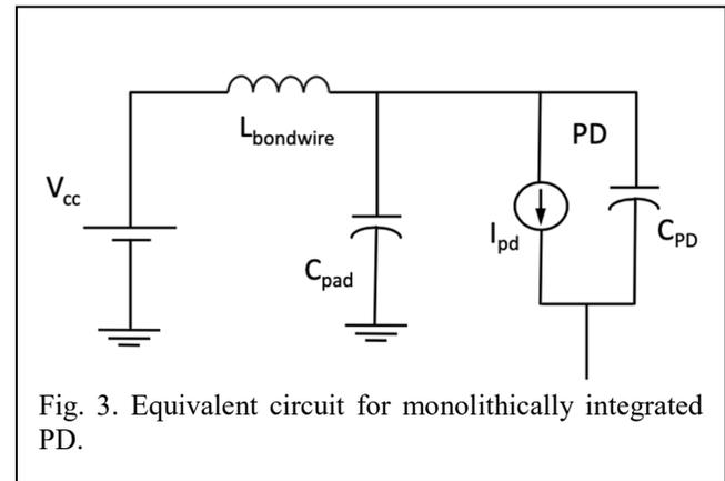
Fig. 3. Equivalent circuit for monolithically integrated PD.
