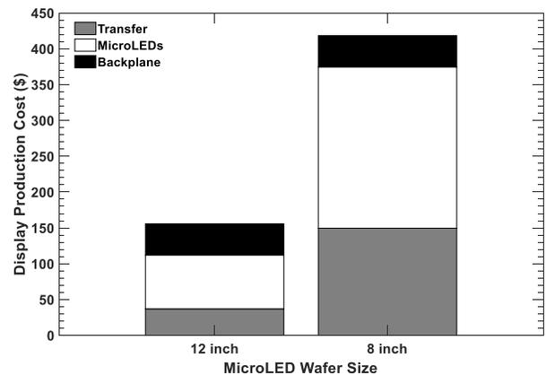
Figure 11. Estimated display production cost for 14" diagonal MicroLED display using "DTM" (a truly massive transfer technology) for 12" and 8" wafers. It is assumed that monolithic RGB is achievable and redundant MicroLEDs per color per pixel [13].
