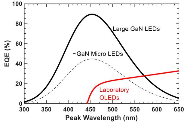
Figure 6. Envelope curves for external quantum efficiency (EQE) versus wavelength for OLEDs and GaN MicroLEDs. Data used to construct the envelope curves are shown in [2].
