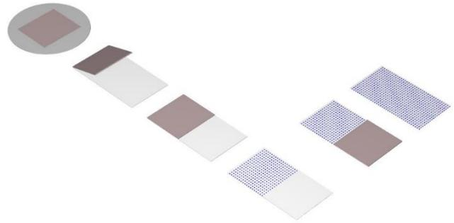
Figure 10. DTM of MicroLEDs from growth wafers directly onto backplane using large stamps [12]. A large stamp from a round wafer is used to stamp backplane, transferring MicroLEDs using the so-called "selective bonding" and "selective release".
