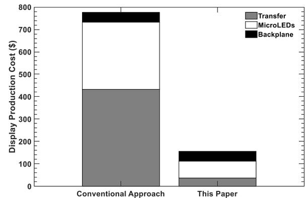
Figure 12. Estimated display production cost for 14" diagonal MicroLED display using current strategy (PnP + 6" wafers + one wafer per color) and proposed strategy ("DTM" + 12" wafer + one wafer per three colors).
