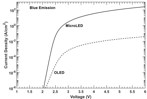
Figure 7. I-V curves for blue OLED and MicroLED. The calculations are based on physics-based models [8]. MicroLEDs have much higher “drive current” compared to OLEDs.
