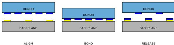
Figure 9. Direct transfer method (DTM) using selective bonding and selective releasing of MicroLEDs directly from their mother wafer [12]. The backplane is populated with copper protrusions that are designed to receive MicroLEDs with copper layer to produce a strong copper-to-copper bonding at high throughput. The laser from backside of the donor wafer is used to selectively de-bond (release) MicroLEDs that have been selectively bonded.
