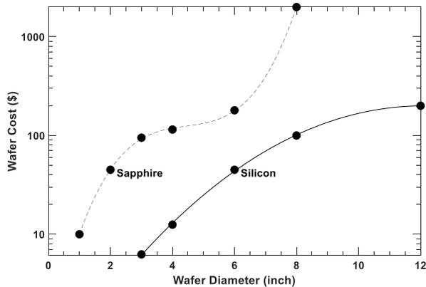
Figure 13. Commercial cost of wafers of sapphire and silicon versus wafer diameter. Silicon wafers are much cheaper than sapphire wafers at a given diameter.
