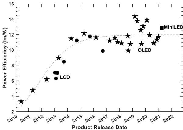
Figure 5. Historical power efficiency of smartphones and laptops with LCDs, OLEDs, and MiniLEDs. The dotted line is guide to the eye. Raw data for power were obtained from www.displaymate.com and analyzed using the methodology published in [2]. The displays had all-white images.
