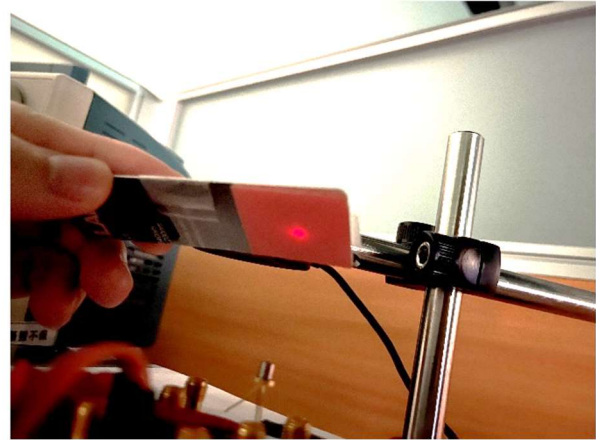
Fig. 5. Illustration of the BHDFB laser beam area using an infrared-band card.
