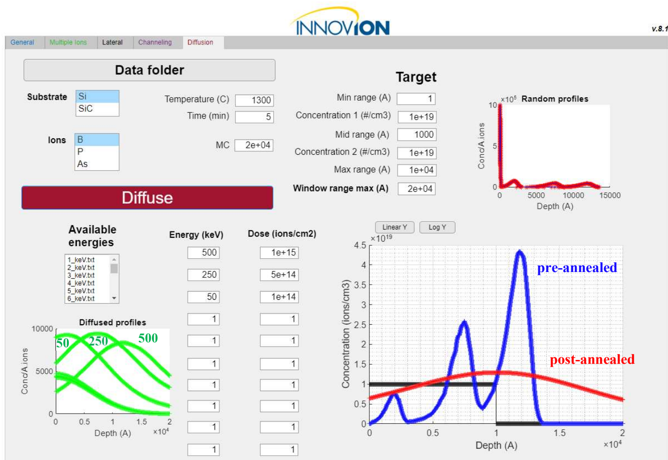
Figure 1. Example of diffused profile of Boron doped Silicon with 3 steps, 500 keV-1e15 ions/cm2, 250 keV-5e14 ions/cm2, and 50 keV-1e14 ions/cm2. The multi peak blue curve is simulated before annealing while the single peak red curve is simulated after annealing at 1300C for 5 min.
