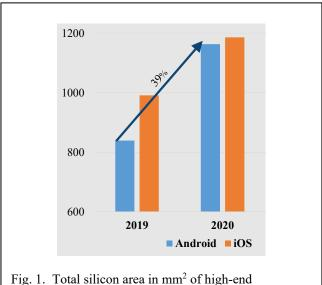
Fig. 1. Total silicon area in mm<sup>2</sup> of high-end smartphones, excluding memory
