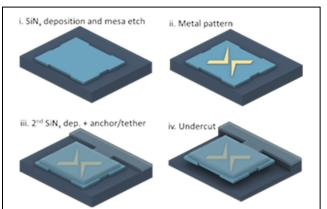
Figure 3: Schematic representation of  $\mu TP$ -compatible 40  $\mu m \times 40~\mu m$  silicon nitride chips fabrication. (i) silicon nitride is deposited and patterned to form a mesa, (ii) thin-film metal is deposited and patterned to serve as an alignment feature, (iii) a second layer of silicon nitride is deposited and patterned to form the anchor/tether system, and (iv) the chip is released by anisotropic etching of the underlying silicon.
