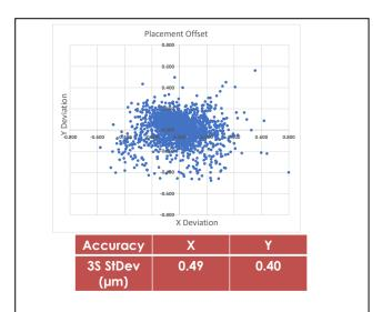
Fig. 9 . 20x28 Array displacement map data for all four prints within 3 sigma for entire dataset.
