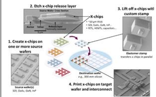
Figure 1: Overview of the MTP process used in an industrial setting.
