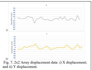
The 2x2 array of test chips provides 30 sets of measurements with 4 printed chips in each measurement, for a total of 120 transferred devices. Test chip placement in the X and Y dimension are shown in Figure 7 with a 3 sigma
