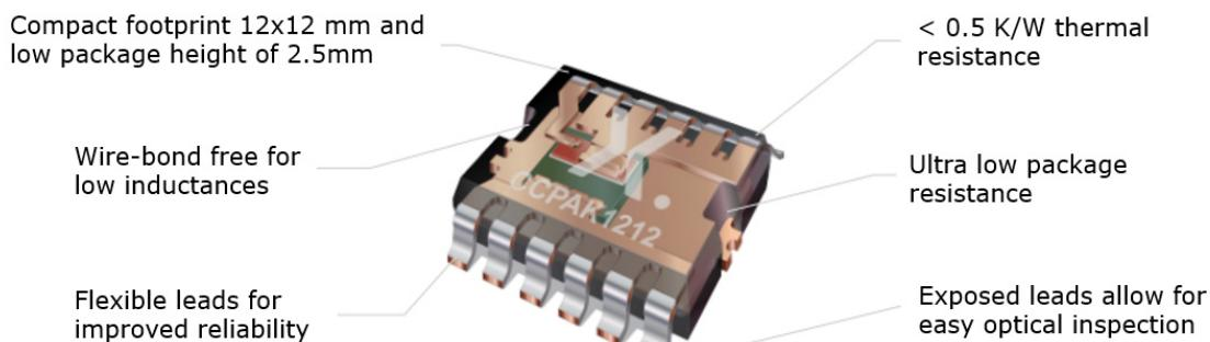
Fig. 1. Skeletal representation of the novel CCPAK Power GaN FETs.
