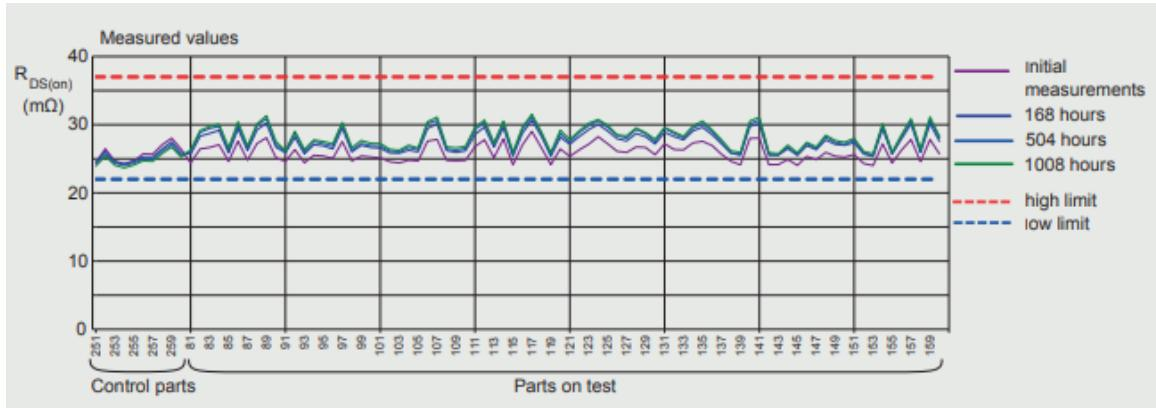
Fig. 4. Dynamic  $R_{DS(on)}$  measurements during HTRB.
