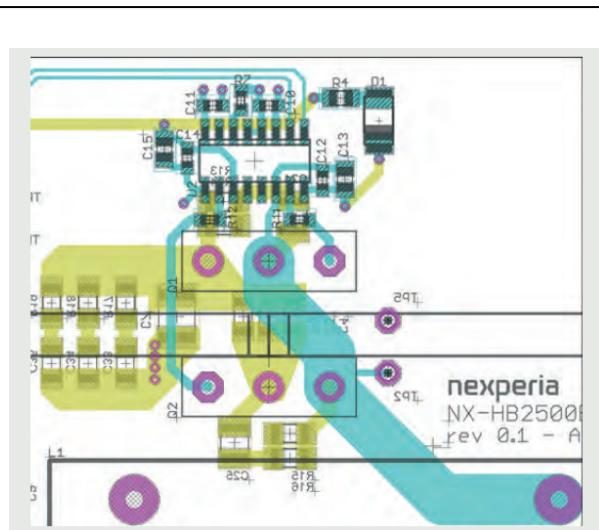
Fig. 5. Portion of a PCB layout of Nexperia's half-bridge evaluation board.
