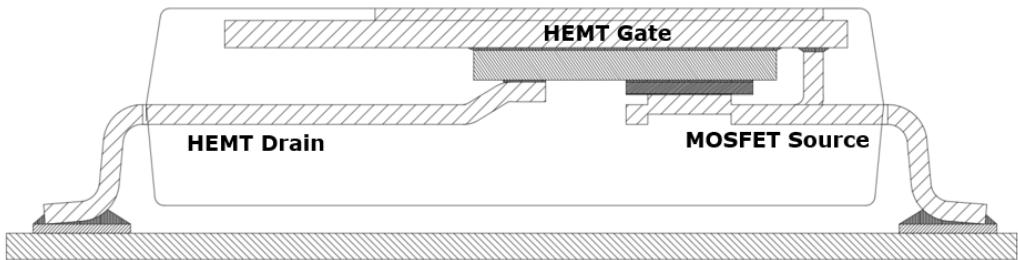
Fig. 3. Top side cooled CCPAK1212.
