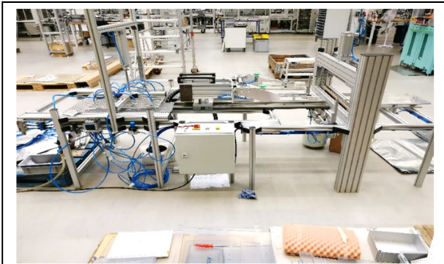
Fig. 5. Demonstrator of a fully automated wafer packaging process.
