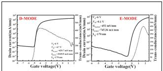
Fig. 5. Transfer curves of the depletion device and normally-off device by ALE etching
