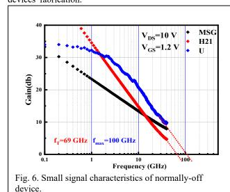
As shown in Fig. 6,  $f_T/f_{max}$  of the normally-off device was 69/100 GHz, with the bias of  $V_{DS} = 10 \text{ V}$  and  $V_{GS} = 1.2 \text{ V}$ , respectively. It was demonstrated that the etching process
