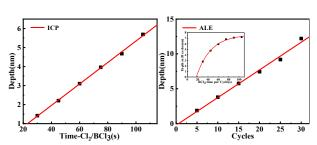
Fig. 3. Comparison of ICP etching rate and atomic layer etching rate
